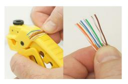
Straighten each wire conductor.
