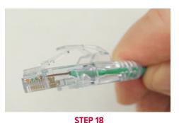
Then remove the terminated RJ45 plug from the crimping socket. Quickly inspect that all wires have been closely trimmed to the plug in the front.
