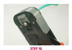
The DT-RJ45-CRIMPTOOL crimper is a ratcheted crimper. The crimper will not open up until the crimping process has been fully completed. This assures that the wire trims and pin sets have been done correctly.
